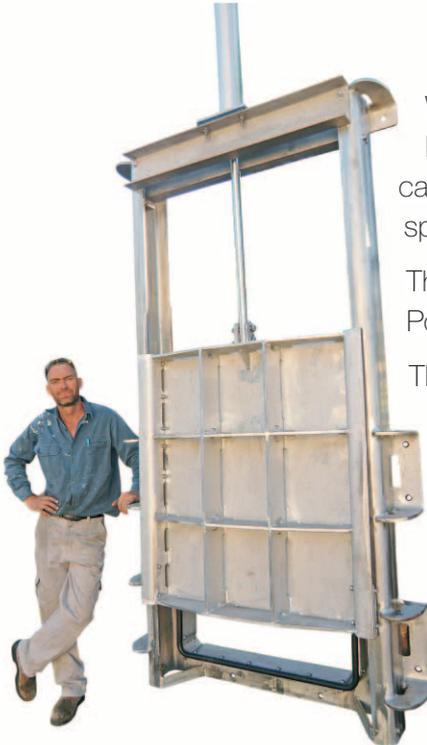
Wedge gates are a type of penstock utilising a whole of gate wedging action. Knife wedge gates are a variation specifically for grit prone invert situations. They can be used for circular or rectangular openings, are drip tight, and designed specifically for the application and duty.
